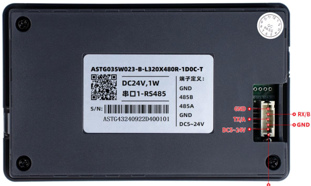
① Power supply interface and communication input interface
